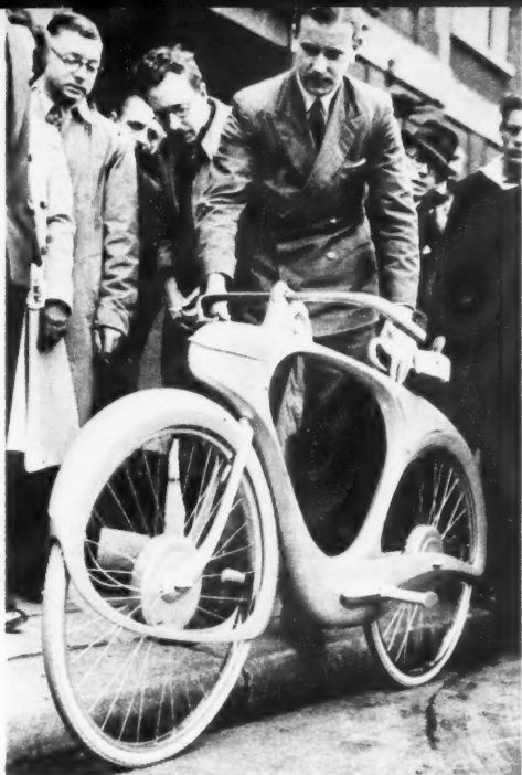
Tomorrow-Cycle is a British-built machine which has a dynamo and motor set storing energy while traveling downhill and releasing it on upgrades. This lightweight oddity was designed by B. G. Bowden of Leamington Spa, England.
